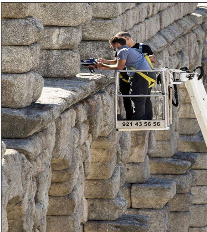
**Fig. 14:** Image of a check-up inspection (special inspection) of the Segovia Aqueduct: two workers from the Spanish Geological and Mining Institute (IGME) take data from granite that makes up the stone ashlars for its geochemical characterization (photograph by Rosa Blanco (VVAA, 2020)).
