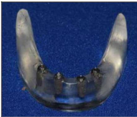
**Figure 1.** Mandibular photoelastic model with four implants placed in the anterior region.
