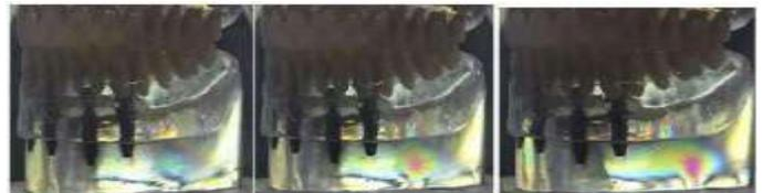
**Figure 3.** Left side view of the photoelastic model with four implants submitted to occlusal force (10, 20 and 30 kgf, respectively).
