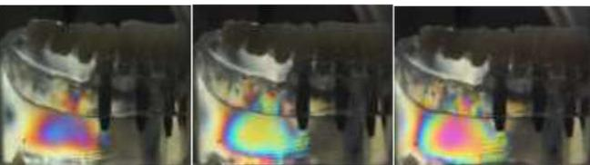
**Figure 6.** Right side of the photoelastic model with four implants submitted to axial single force on the first right molar (10, 20 and 30 kgf, respectively).
