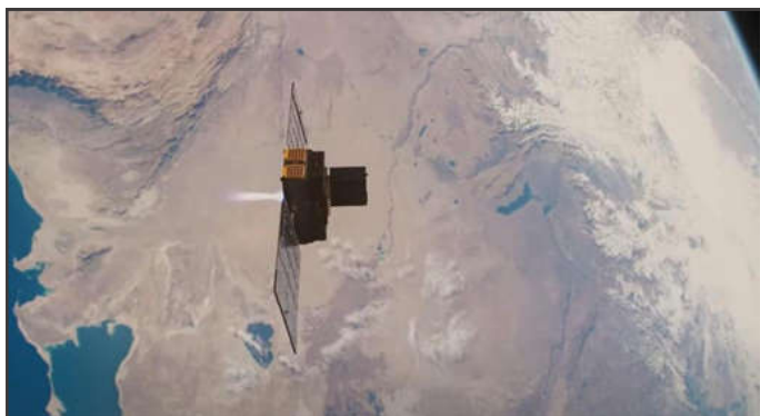
Figure 2. The Vigoride 5 vehicle propelled by the MET thruster using water propellant.
