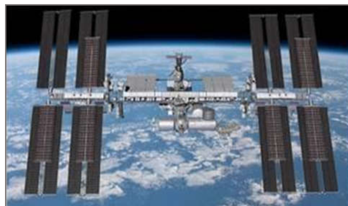
Figure 8 The 215 kW Solar Power arrays of the ISS.
