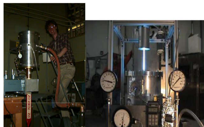
Figure 6 The 75kW MET thruster using water vapor propellant. The 75kW MET operates on 915MHz Microwaves that can generated with 95% efficiency.
