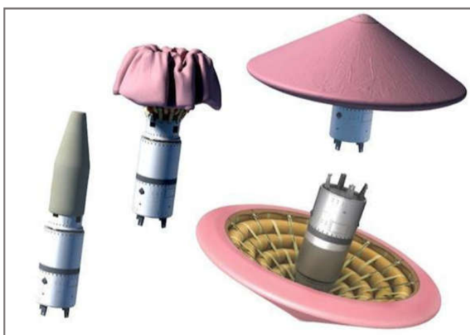
Figure 3 the Inflatable Aerobrake Shield
