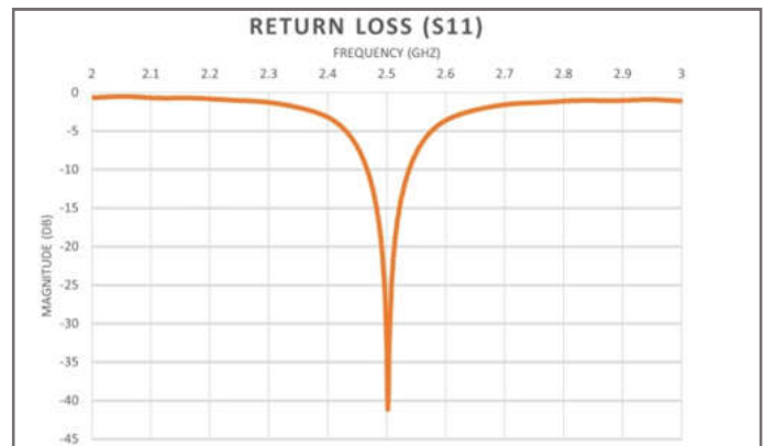
Fig. 2. Power Reflection Coefficient–S1,1 of Antenna
