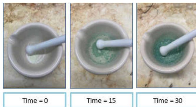
Figure 6: Mechanochemical synthetic approach to eliminate use of solvent and reflux during step 3 of the student reaction
