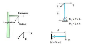
The forces on monopod supports are determined by the choice of active conductors, and are generally provided by customers and calculated in accordance with national standards. they can also be given in two ways: by editing a tree of mechanical loads (vertical, horizontal and transversal forces) directly entered into a calculation program.
