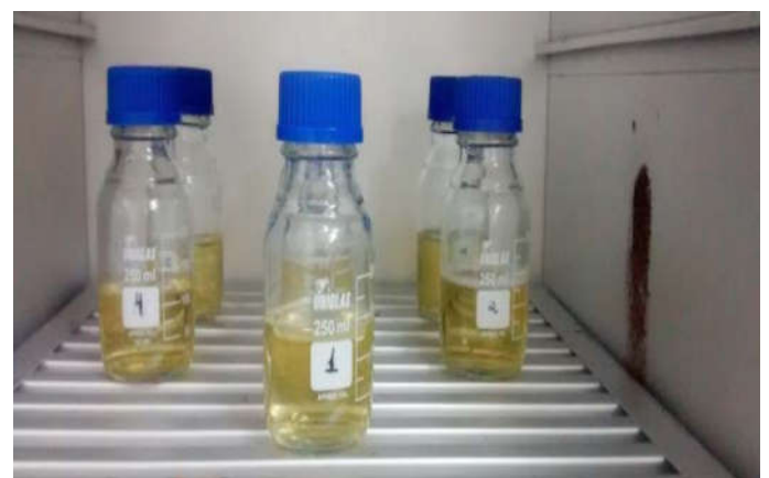
Fig 2. Water samples in the incubator at 37°C
