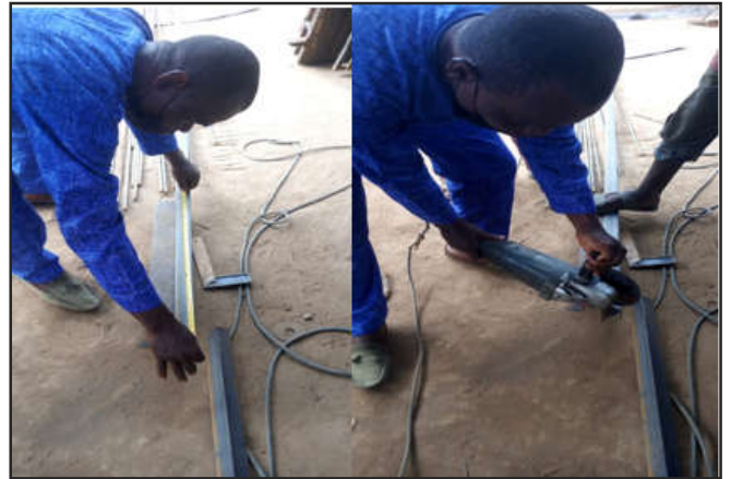
Figure 2a. Measuring angle bar for chassis frame (Ejiogu, 2021) Figure 2b. Cutting of flat bar for chassis frame (Ejiogu, 2021)
