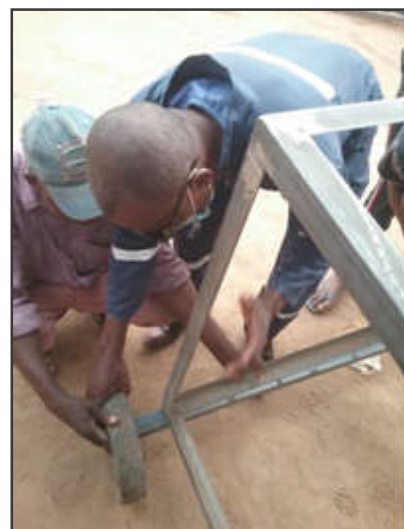
Figure 3b. Fixing of tyre with the axle via the hub (Ejiogu, 2021)
