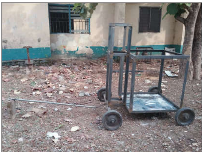
Figure 4a. Complete mobile chassis for brick-built kiln (Ejiogu, 2021)
