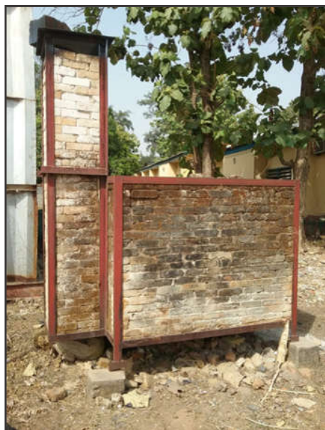
Figure. 1. Suspended brick-built static kiln in the FCT College of Education Zuba-Abuja. Department of Fine and Applied Arts (Ejiogu, 2021)
