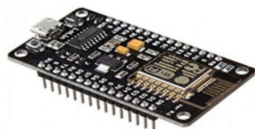
Fig. 3: NODEMCU - ESP8266 WiFi Development Board
